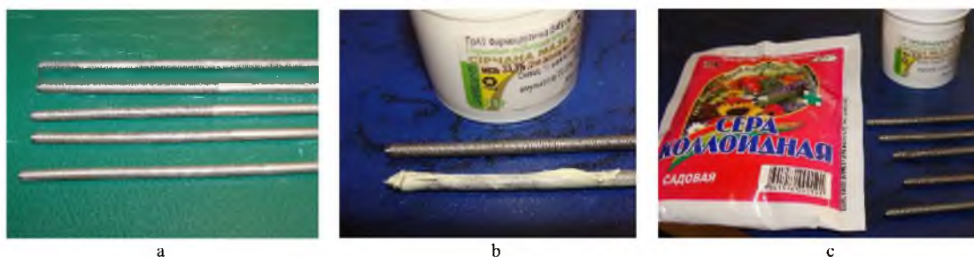
Fig. 1 – The electrodes are made of 12X18H10T (12H18N10T) stainless steel Ø 3mm intended for sulphiding the parts by EEA method
