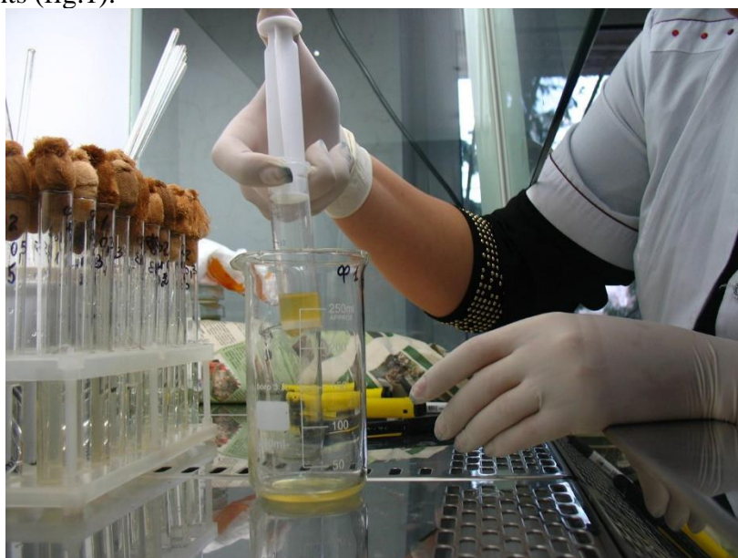
Fig. 1. Separation of the culture fluid of P. aeruginosa using filtration through a porous filter element based on fluoroplastic in the laminar box
