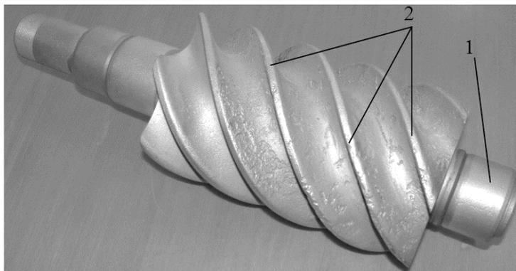
Fig. 1 – Characteristic regions of wear of the rotors of a screw compressor:
