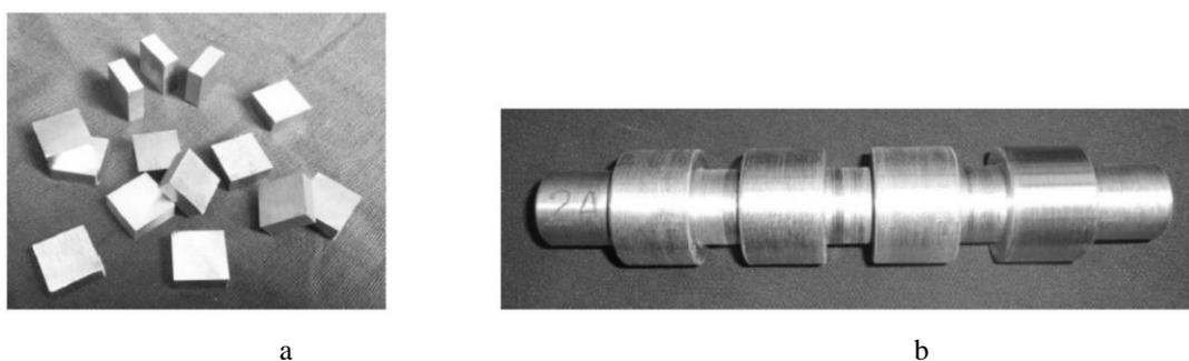
Fig. 2 – Flat (a) and round (b) specimens produced from steel 40
