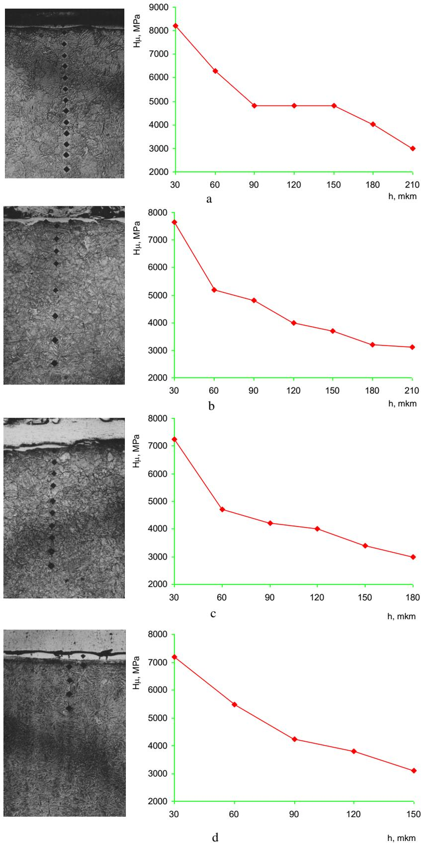
Fig. 4 – Microstructure and distribution of microhardness of surface layer of specimens of steel 40Kh following treatment by IN + EECA with partial removal of the hardened surface layer following ion nitriding to a depth of: a – 0.05 mm; b – 1.0 mm; c – 0.15 mm; d – 0.20 mm.
