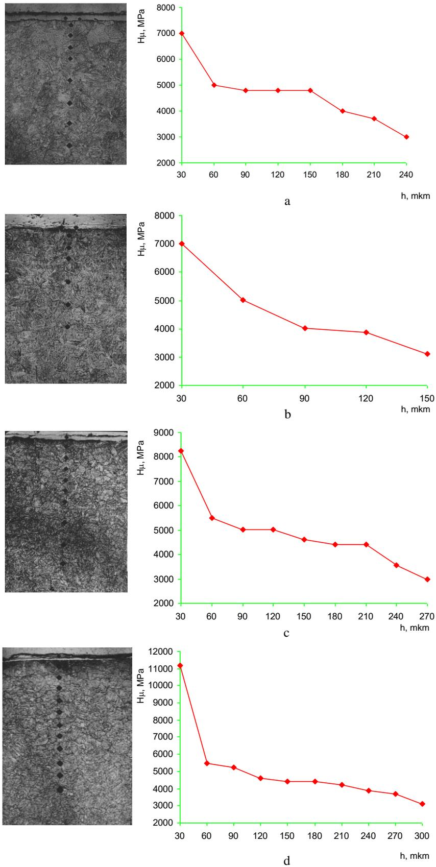
Fig. 3 – Microstructure and distribution of microhardness of surface layer of specimens of steel 40Kh following treatment: a – IN; b – EECA; c – EECA + IN; d – IN + EECA.
