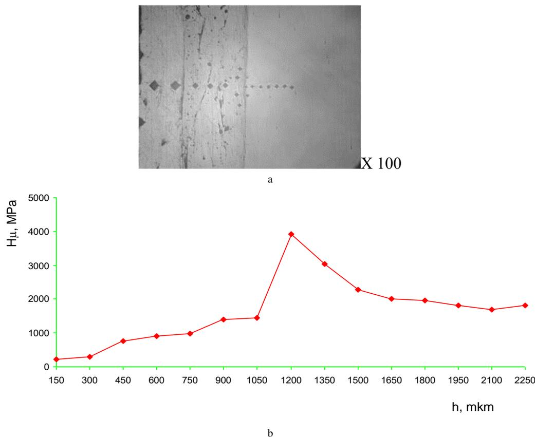
Fig. 6 – Structure (a) and distribution of microhardness by depth of layer (b) following treatment by electroerosion alloying of steel 40 on a EIL-9 plant with bronze and babbitt B88.
