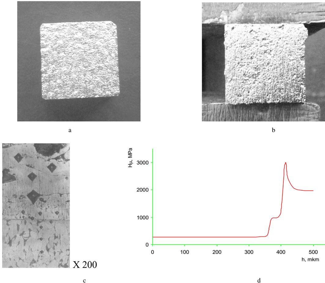
Fig. 5 – Sample of steel 40 following treatment by electroerosion alloying of bronze (a), bronze and babbitt B88 (b), structure of the coating (c), and distribution of microhardness by depth of layer (d).
