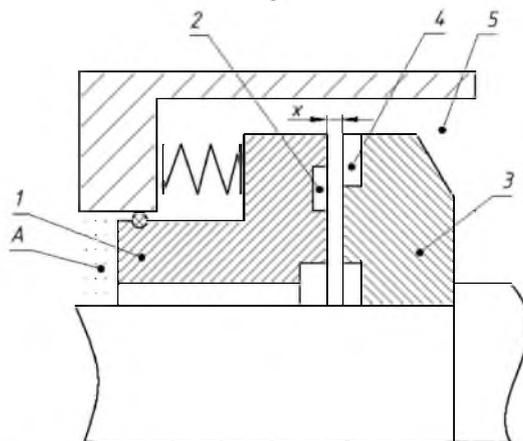
Fig.1 – Traditional schematic construction of face impulse seal
