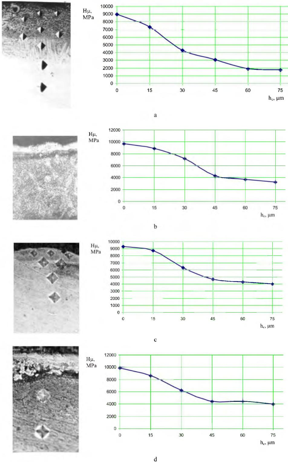
Fig.7 – Structure and distribution of microhardness over the depth of the layer of 12H18N10T (a), 38H2MUA (b) steel grades and HN58MBUD (c; d) alloy samples after: CEEA and EEA WC8 + Cu + WC8 (a, b); EEA WC8+WC8 + Cu (c) and EEAWC8+WC8+Ni (d)
